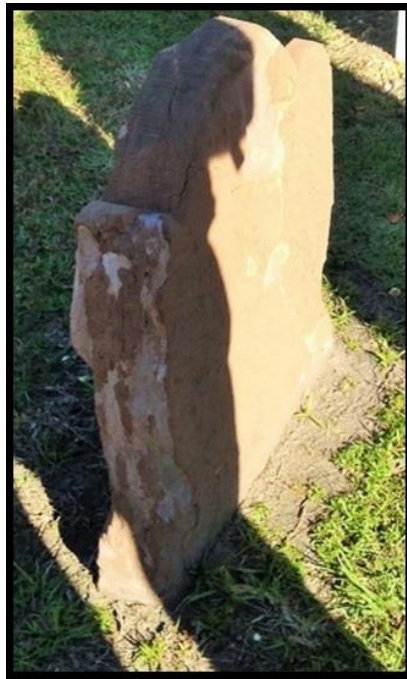
Savannah, Georgia, brownstone tombstone where an example of case hardening can be seen 113
