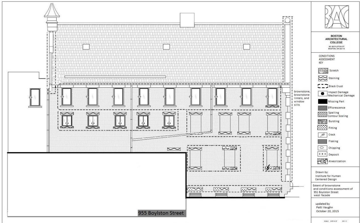
951 Boylston Street, west façade, extent of brownstone and conditions assessment
